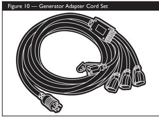
The maximum load on each outlet is 20 Amps. The maximum total load on both yellow wire outlets or both black wire outlets is 30 Amps.
